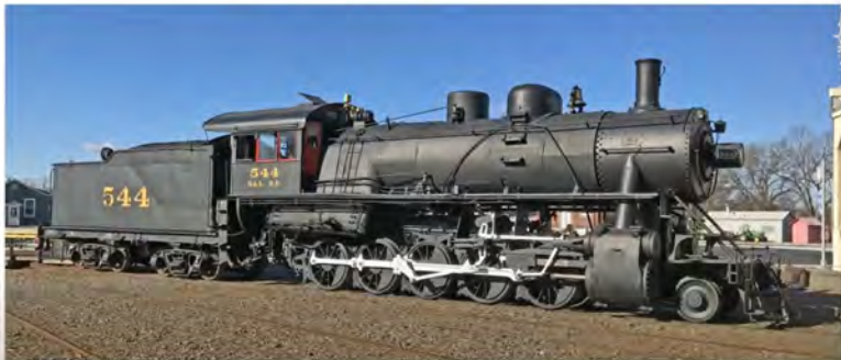
Seaboard 544 (Alco serial no. 58902), a Russian Decapod, is cosmetically restored at the North Carolina Transportation Museum in Spencer, NC. Photo: H. George
