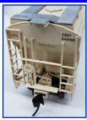
looked at. The crossover platform on each end of the car does appear to be lacking in detail as it is cast on rather than a separate casting.
