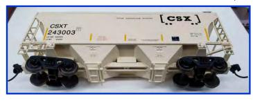
center sill car, optimized for transporting cement, sand, or other high-density products. The car features round side and roof construction, multiple hatch options to meet specific shipper needs and a high side sill for easier access to outlet gates and vibrator brackets." (www.progressiverailroading.com/railproducts/product/3281-Cubic-Foot-Covered-Hopper--75)
